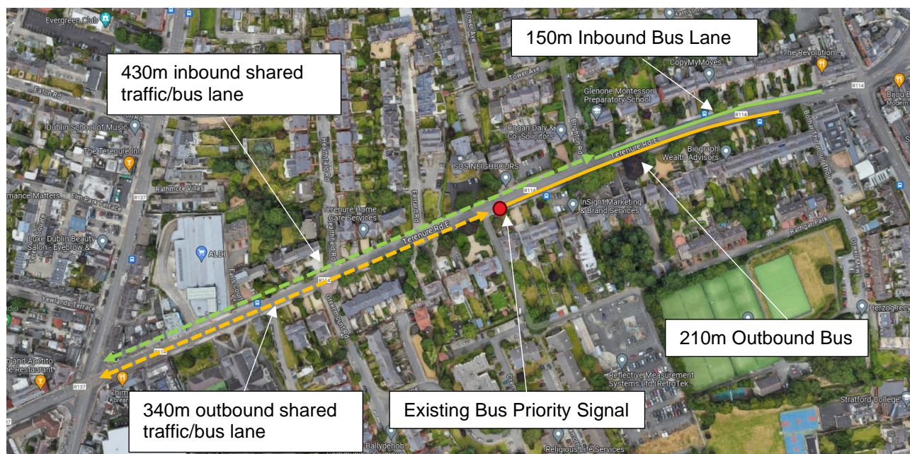
Figure 2.4.23 Existing Arrangement on Terenure Road East
