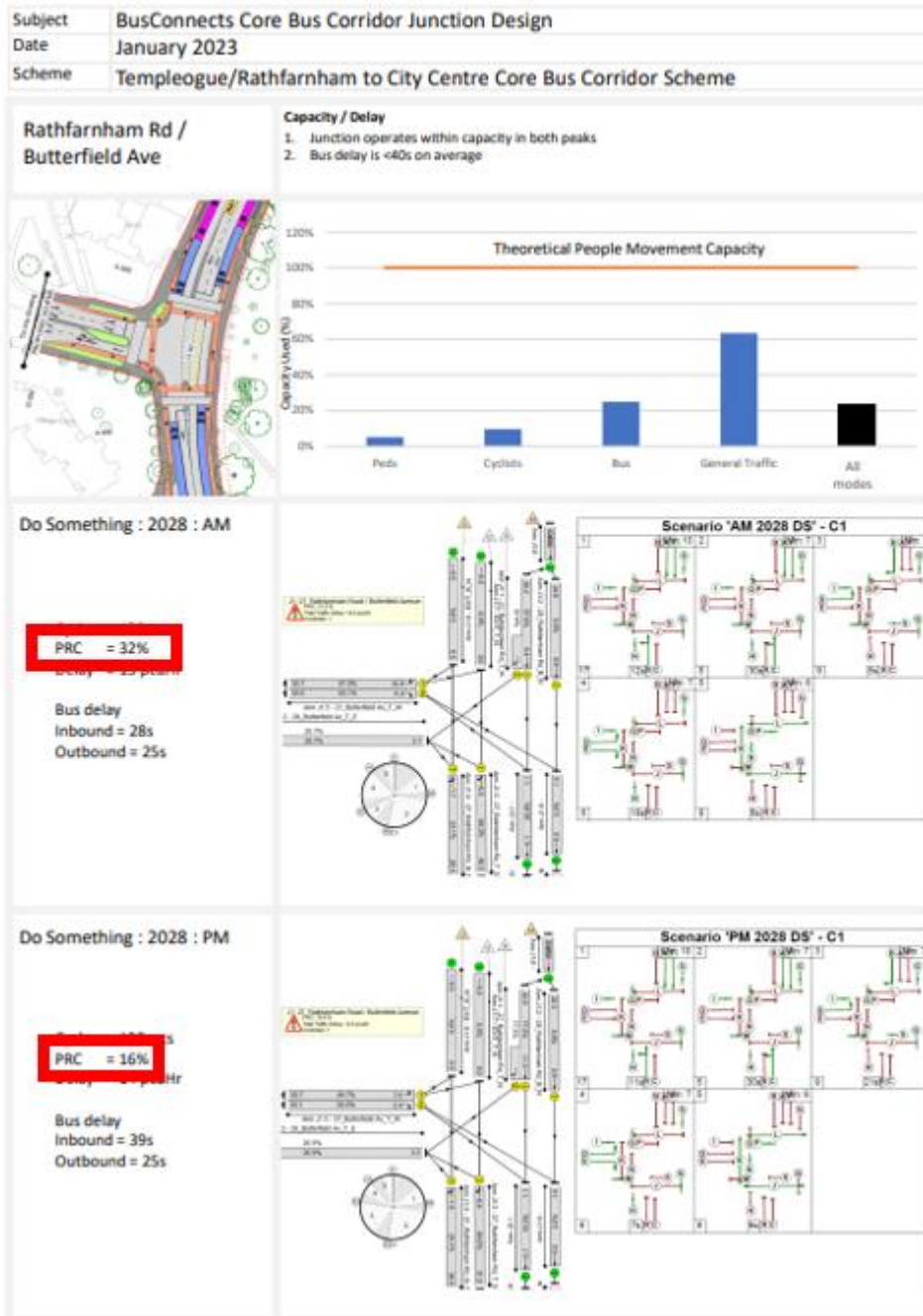
Figure 3.63.25 Extract from junction design report showing Practical Reserve Capacity (PRC) at Rathfarnham Road/Butterfield Avenue junction.
